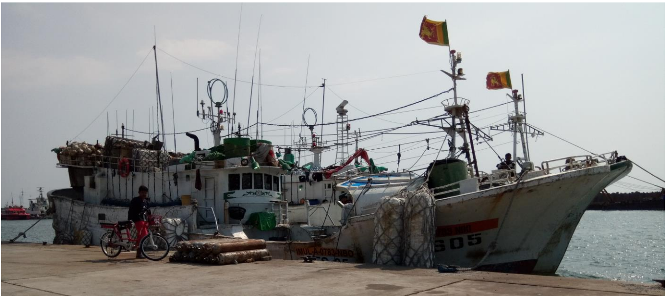
Figure 2: Industrial (>24m) Sri Lankan flagged Large Scale Tuna Longline Fishing Vessel (Image credit Steve Creech).
